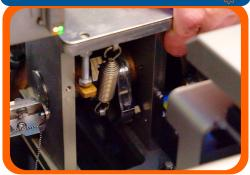
Engineered for easy maintenance, the knotting head can be removed in minutes with just four bolts.
